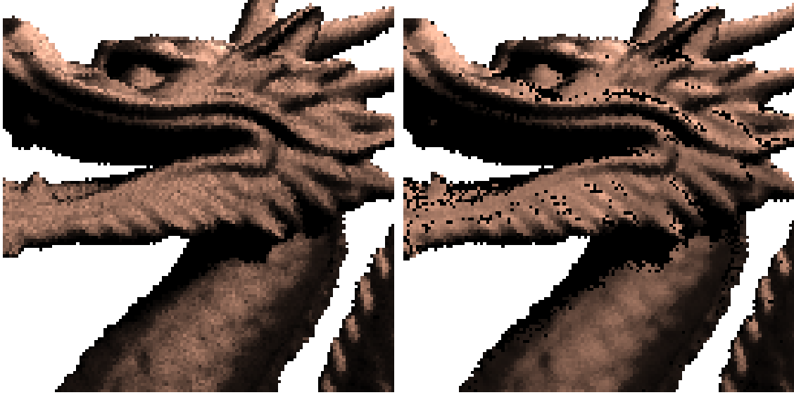
Figure 5.1: Dragon sampled with a single primary ray and using RIS with different values of M and N to compute direct lighting (in equal time). On the left, N = 20 , M = 20 and on the right N = 1 , M = 60 . The right image has less variance except where visibility is a major component of the variance.
